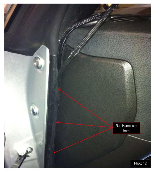
Warning: Ensure there is no excess harness that may interfere with the pedals. You may need to pull some of the FST10-UNI harness back into the engine bay to eliminate slack in the cabin.
