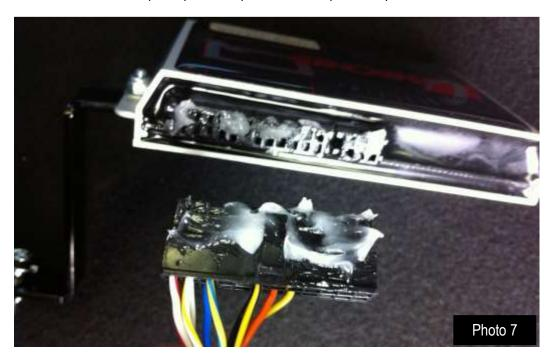
e. Connect the black 24-pin StS Plug *Unichip* into the large Unichip Computer connector.
